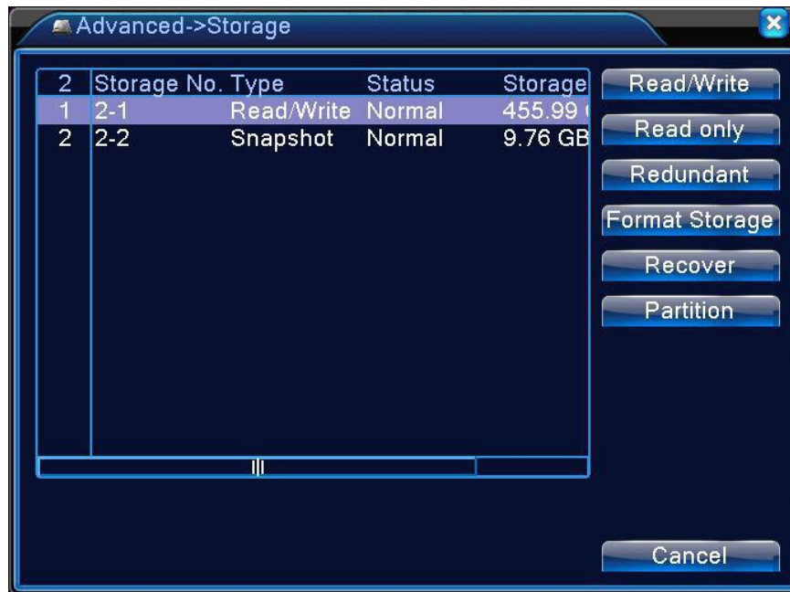
Pic 4.40 HDD manage
