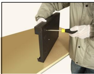
④fix the screw of hard disk
