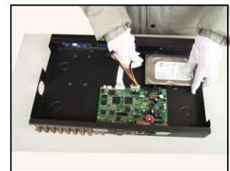
⑥connect the power wire
