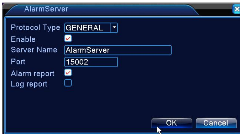
Alarm server setting
