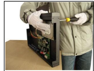
③fix the screw of hard disk
