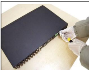
①disassemble the screw
